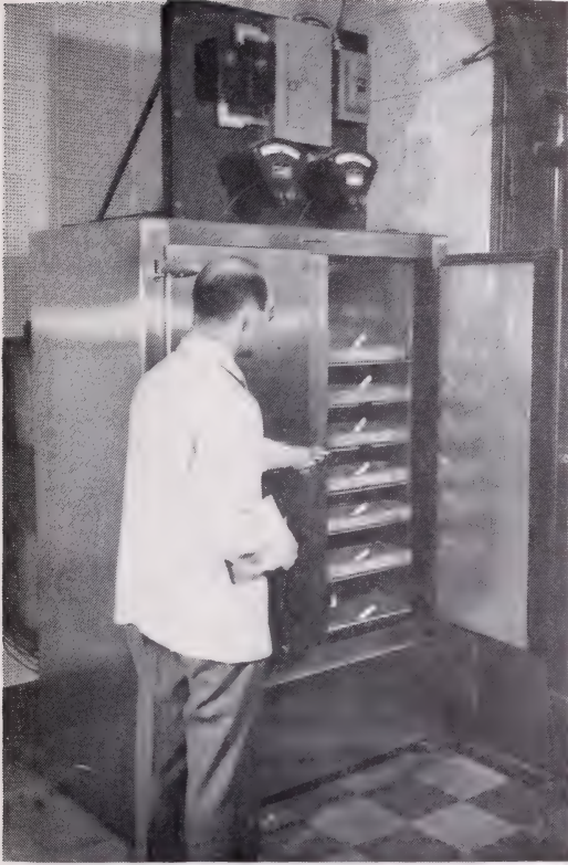
Apparatus for cold-testing seed corn under conditions approximately those of early spring in the field.
